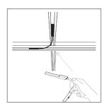
ELECTRICAL CONNECTION Every T-Connector is enclosed with one, every X connector with two flexible cross adapters. An electrical connection of the pieces can be established with these components with ease.
