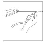
TRACKMASK A black flexible rubber cover, easy to cut directly on site after positioning the inserts and integrated inside the track, is the final touch to furtherly minimize the appearance of the MINIMAL TRACK.
