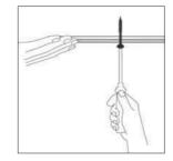
TRACK MOUNTING The track is conceived to be easily cut on site, and directly screwed to the ceiling for a tailor-made result in each installation.
