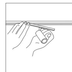
**INSERTS** Place and remove any insert wherever you want by simply pulling it out and snapping it in without any tools needed.
