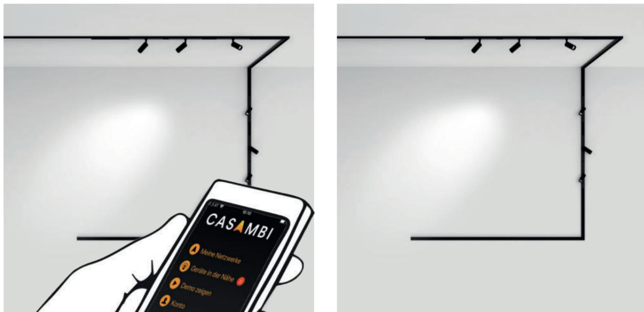
Despite its exceptionally compact size, the MINIMAL TRACK is designed as a DALI track that can be integrated into any lighting control system. It has two conductors dedicated to DALI in order to enable completely individual control of each installed luminaire.
