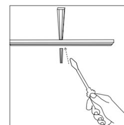
**CROSSINGS** Complex connection pieces belong to the past with MINIMAL TRACK. The linear elements can be used to create crossings in the easiest way. Even after the installation, adaptations can be made with minimal effort.
