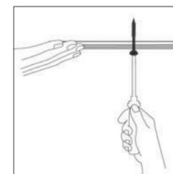
**TRACK MOUNTING** The track is conceived to be easily cut on site, and directly screwed to the ceiling for a tailor-made result in each installation.
