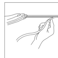
**TRACKMASK** A black flexible rubber cover, easy to cut directly on site after positioning the inserts and integrated inside the track, is the final touch to furtherly minimize the appearance of the MINIMAL TRACK.
