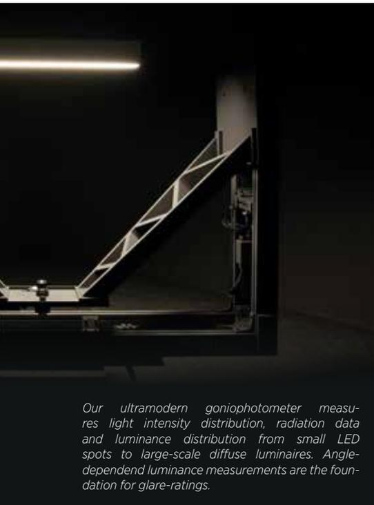
*Our ultramodern goniophotometer measures light intensity distribution, radiation data and luminance distribution from small LED spots to large-scale diffuse luminaires. Angle-dependent luminance measurements are the foundation for glare-ratings.*
