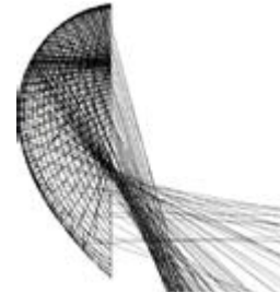
Each facet of the Bartenbach RDB reflector provides broad and clean illumination without multiple shadows.
